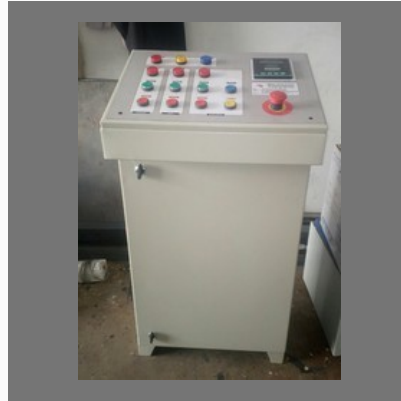
Slitting Machine Panel
